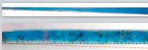
▲ Figure 5 Side view of our shelf. Theory predicts the apparent discrepancy in the middle, where the gradient exceeds that near the source (right) – this should cause a variation in velocity along the tank.
